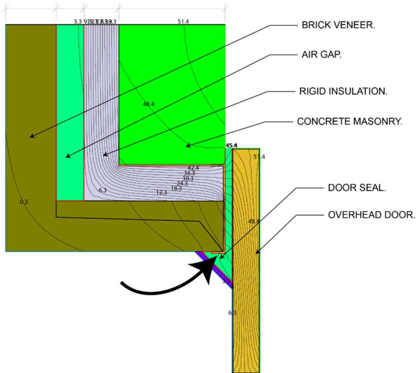
*Model (2B): Overhead garage door, improved jamb detail.*
