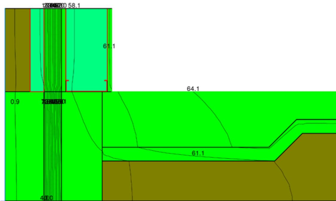
Model (6C): Thermally broken foundation.
