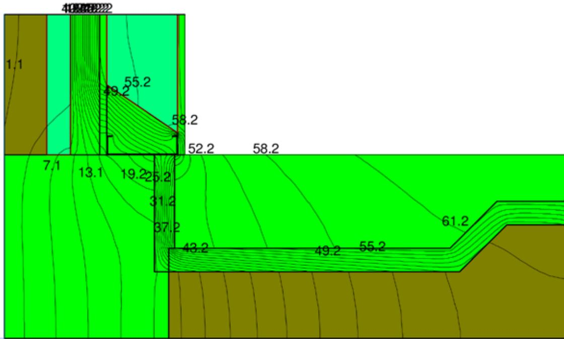
Model (6B): Increased insulation between slab and foundation wall.
