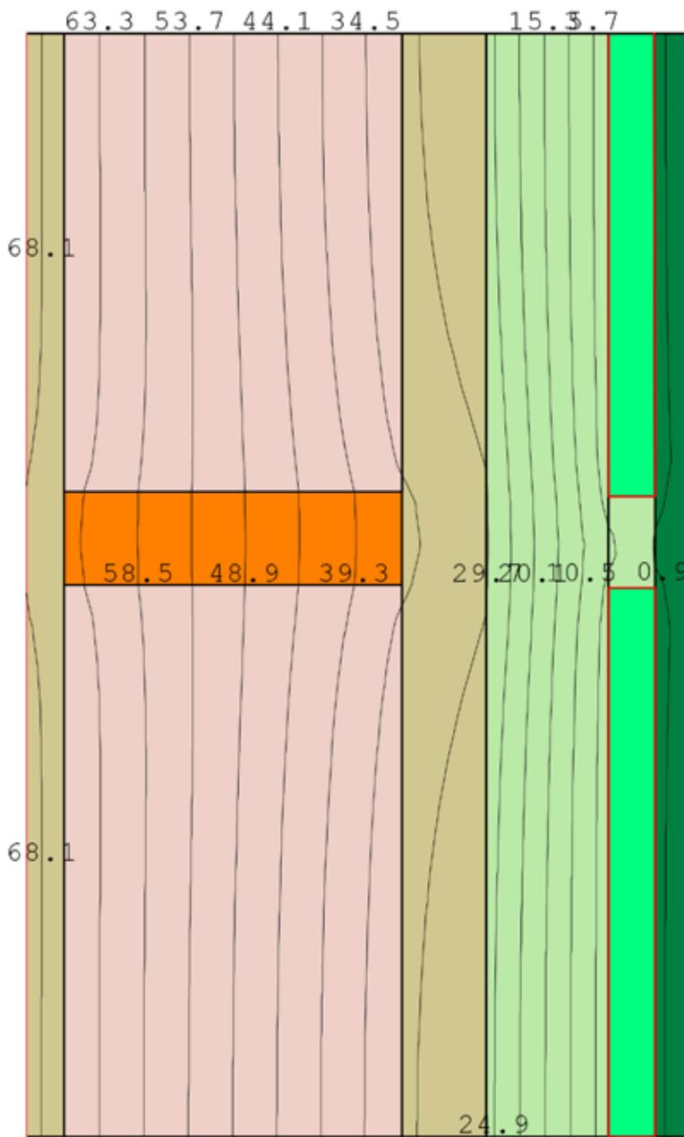
*Model (5B): Continuous insulation added to existing wood framed wall. R-value = 32.*
