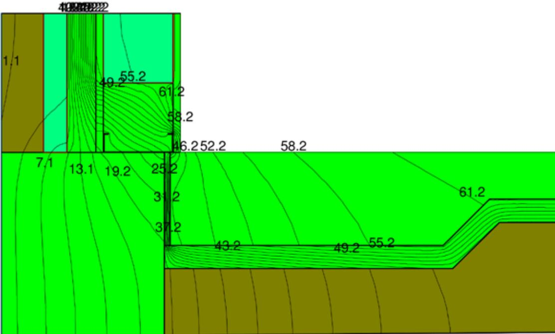
Model (6A): Base case metal stud backed veneer brick on concrete foundation.
