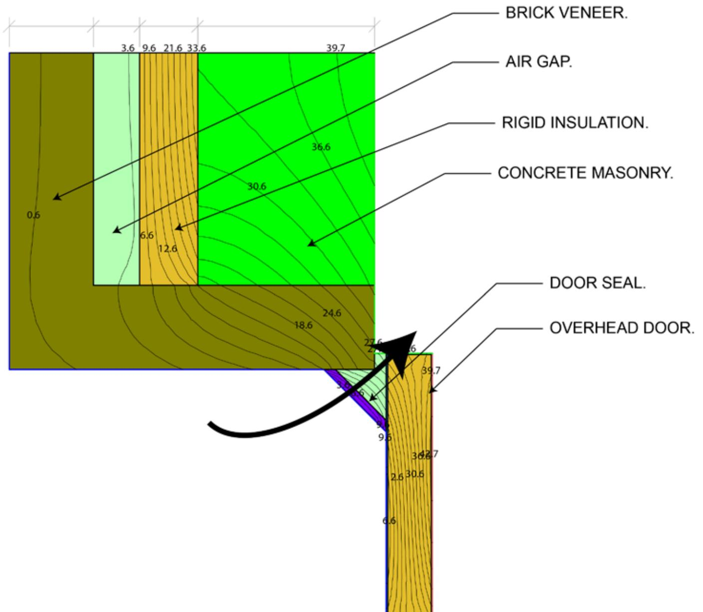
*Model (2A): Overhead garage door, typical jamb detail.*
