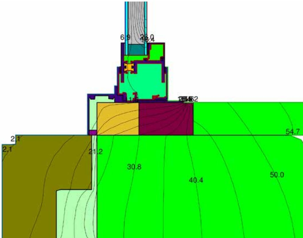
Model (1A): Uninsulated brick and concrete masonry wall.
