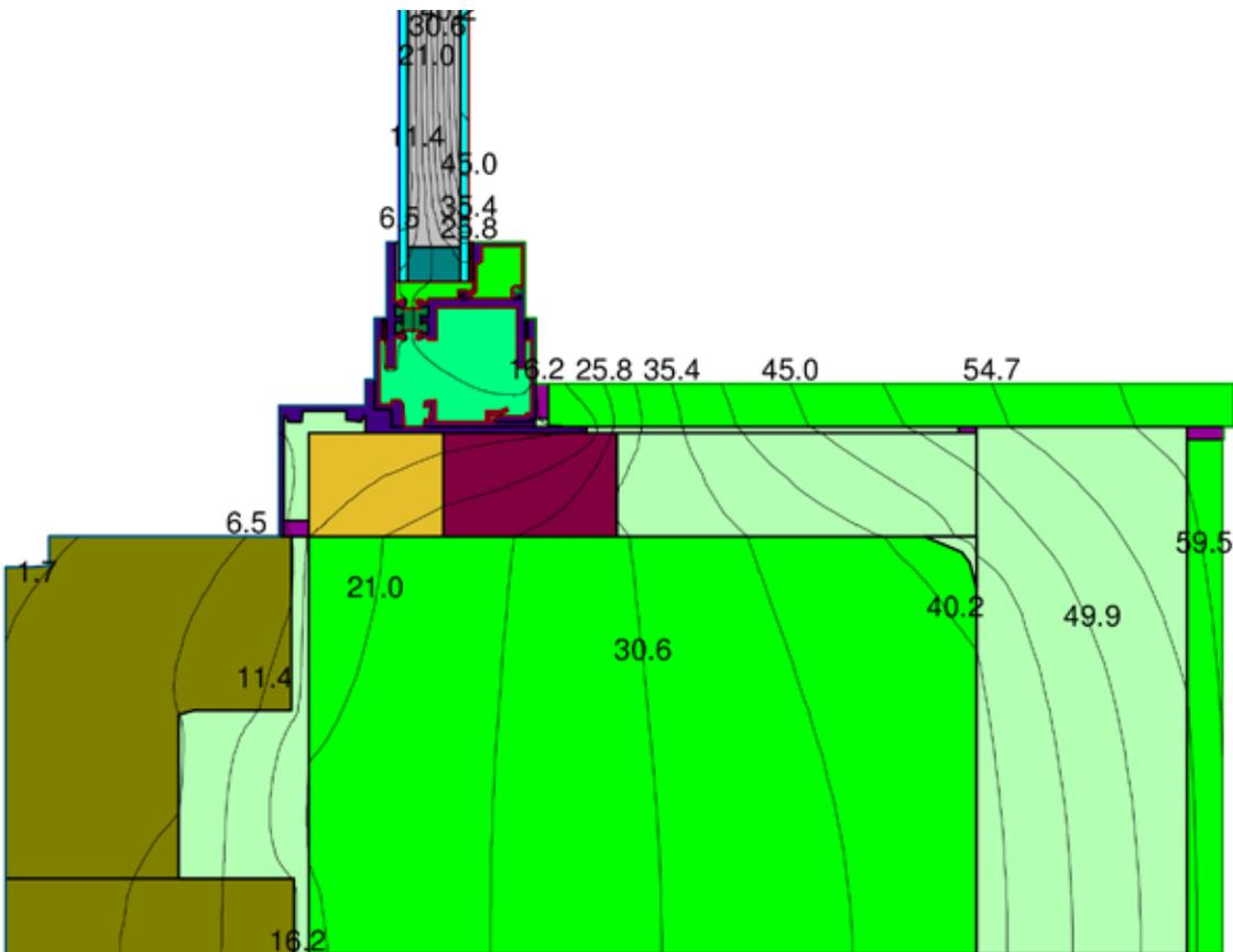
Model (1B): Frame cavity (no insulation) on interior side of exterior wall.
